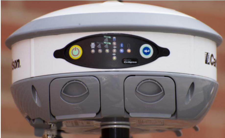
It utilizes the Eclipse (TM) II OEM Board from Hemisphere. Each receiver comes with a kit of accessories as outlined below:
