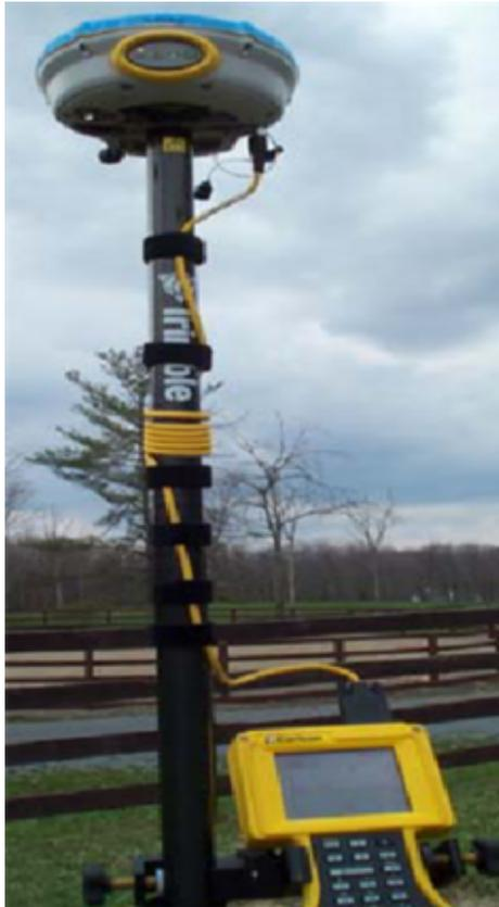
The Trimble 5800 with Zephyr antenna has a panel that includes an On-Off button at right.
