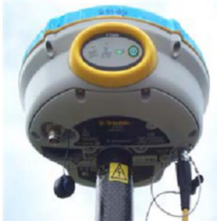
There are three LCD lights. From left, the first round light is yellow and flashes or pulses at 1 per second when sufficient satellites have been acquired for RTK, and flashes quickly when insufficient satellites are available. The second round light is a pulsing green light indicating radio linkage. When the pulse is intermittent, radio connection is being interrupted. The third, rectangular light is green and indicates battery status. It is steady on when there is sufficient battery power.
