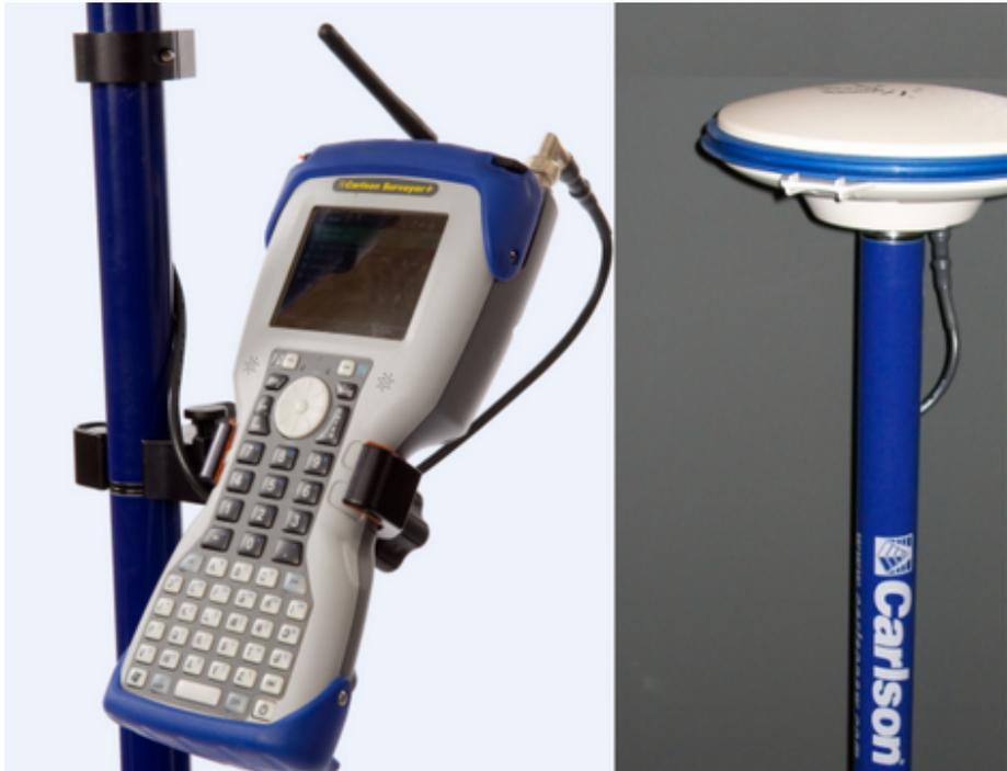
The Surveyor+ GPS system is specially designed for use as a rover with GNSS reference systems such as Trimble VRS, Leica Spider, Topnet, Geodetics or Geo++. Communication is typically by cell modem. Note the two LED lights above the circular arrow key button, just below the screen. The LED on the right blinks steadily when corrections are being received.
